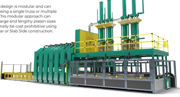
Similar to a Tie Bar press, a system of gibs are used to maintain parallelism and squareness of the working surfaces. Gib-quided presses are uniquely suited to endure the rigors of the most demanding applications.
