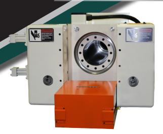
For over *30 years,* Trinks Inc. has been the leading supplier of Lithium Extruders. This machine is used to shape lithium ingots by forcing them to flow through a shaped die to create lithium foil.
